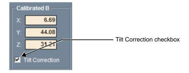
The eCompass will still operate if it is held flat, but pitching or rolling the device will cause dramatic compass heading errors.
