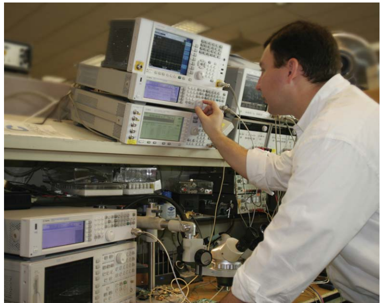
Express MXG analog signal generators cover a wide range of applications including local oscillator (LO) and clock substitution; continuous wave (CW) interferers; power calibration; antenna testing; and analog communication systems that use AM, FM or phase modulation.
