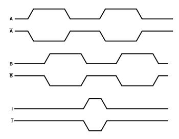
Waveforms for Encoders with Line Drivers.
