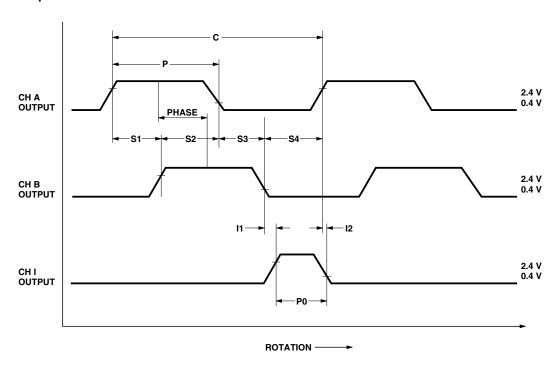
**Waveforms for Encoders without Line Drivers.**
