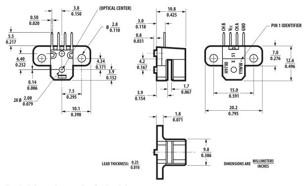
Mounting Option #51 – Screwmount (Baseplane Mounting)
