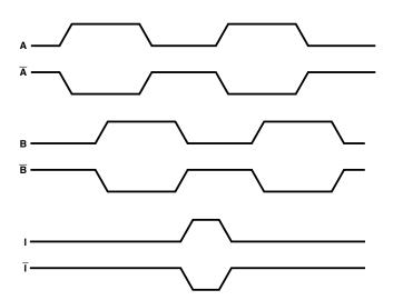
**Waveforms for Encoders with Line Drivers.**
