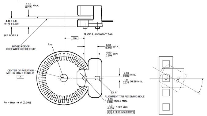
For linear motion, angular misalignment, EA, must be  $\leq \pm 2$  degrees to achieve Encoding Characteristics. All dimensions for mounting the module and codestrip should be measured with respect to the two mounting posts, shown above.
