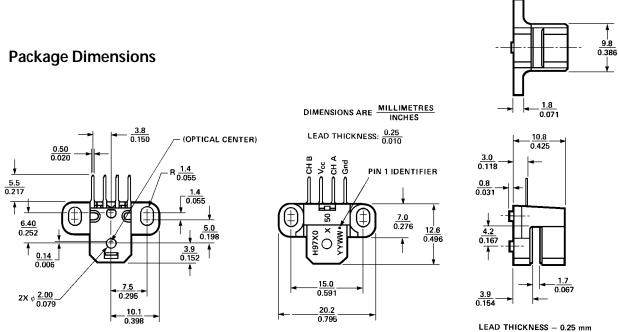
LEAD THICKNESS – 0.25 mm LEAD PITCH – 2.54 mm
