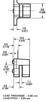
Mounting Option #50 - Standard (Baseplane Mounting) Contact Factory for Detailed Package Dimensions
