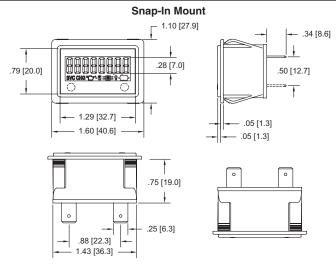
Panel Cutout: 1.46" [37mm] x 0.95" [24.1mm] Minimum Panel Thickness: 0.04" [1.0mm] Maximum Panel Thickness: 0.125" [3.18mm]
