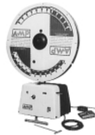
AMP-TAPEMATIC Stripper/ Crimper Machine Part Number 599406-7
