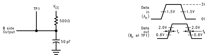
FIGURE 4. A to B Direction Test Load and Waveforms for Open Drain B 1 - B 7
