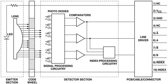
There are two different connector pin-out configurations used with the HEDS-65xx / HEDL-65xx series of encoders. The table below relates the part to its connector pin-out.
