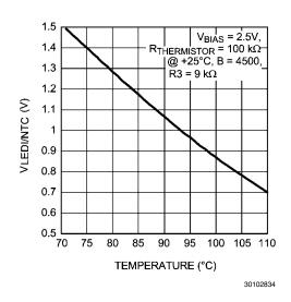
FIGURE 20. Thermistor Resistive Divider Response vs Temperature
