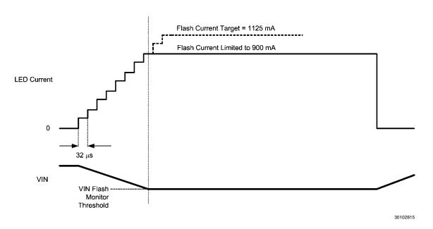
FIGURE 12. VIN Flash Monitor Example
