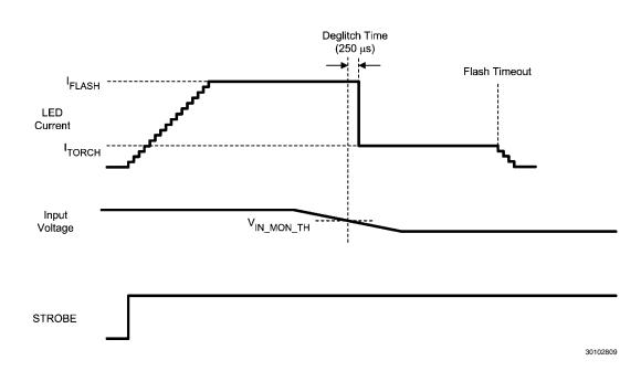
FIGURE 11. VIN Monitor Waveform
