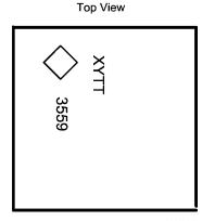
16-Bump 1.97 mm x 1.97 mm x 0.6 mm micro SMD Package TLA16 XY (Date Code), TT (Die Traceability)
