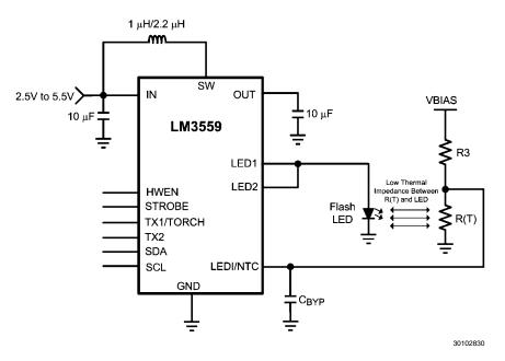
FIGURE 19. LM3559 Typical Application Circuit with Thermistor
