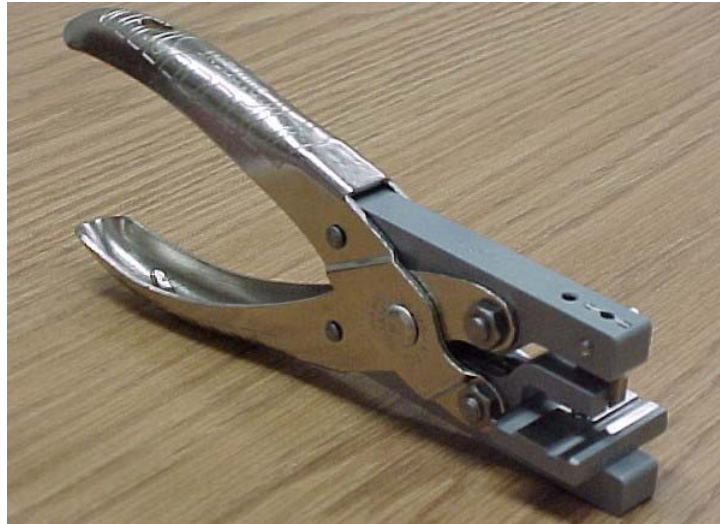
Figure 24 BPY75D37 Wire Insertion Repair Tool
