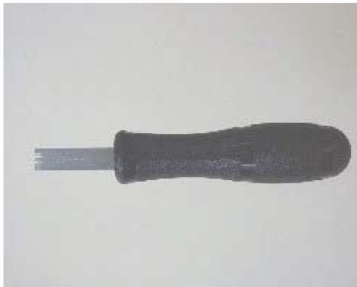
Figure 24 BPY75D37 Wire Insertion Repair Tool
