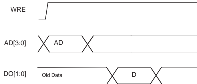
Figure 3-7. Slice Single /Dual Port Read Cycle Timing
