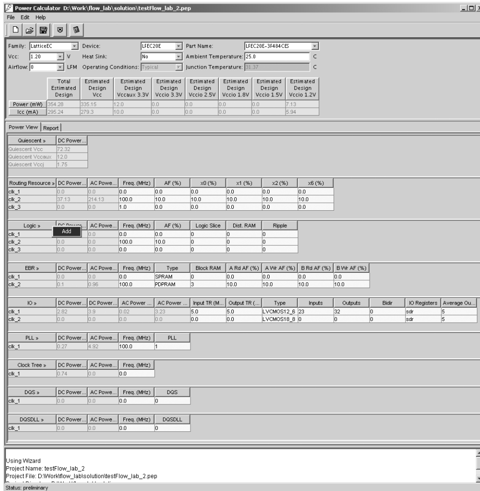
Figure 12-14. Power Calculator Main Window – Adding Resources
