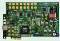
The LatticeECP3 Serial Protocol Board provides a platform to evaluate the LatticeECP3 device's multi-protocol serial protocol functionality as well as DDR2 and DDR3 memory interfaces.
