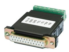
72-CNV-4 and 72-CNV-5 convert serial communications from RS-232 to RS-485 in both directions. The converter simply plugs into any male RS-232 DB-25 connector and converts the transmit and receive signals to RS-485 (RS-422) levels at speeds to 115.2 KB. The converters are configured for DTE (default) or DCE operation.
