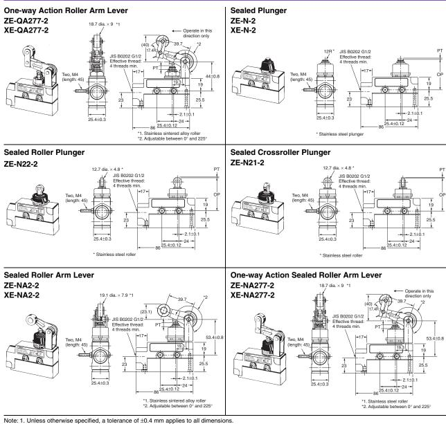
2. The diagrams shown the Switches with two, M4 screws (length: 45) attached. (The screws are provided.)
