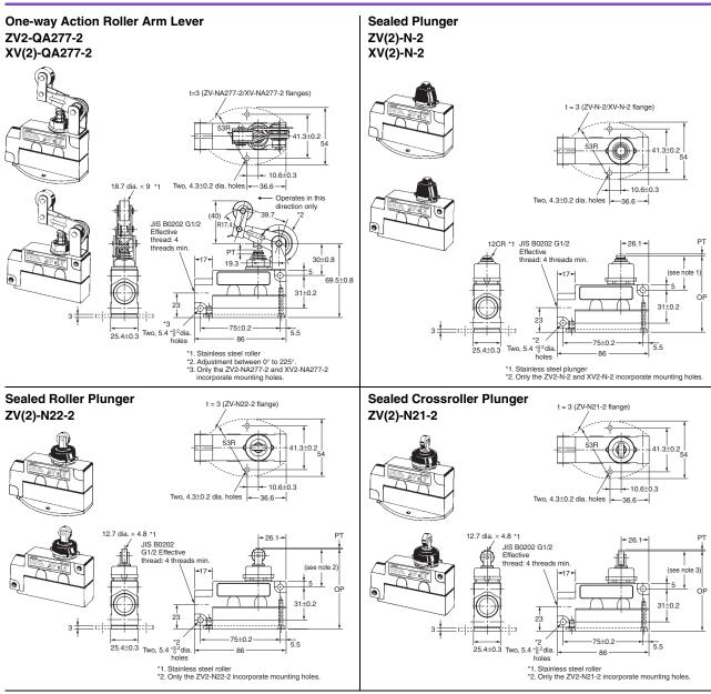
Note: Unless otherwise specified, a tolerance of ±0.4 mm applies to all dimensions.
