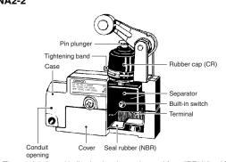
Note: The conduit thread indication has been changed from "PF1/2" to "G1/2" accompanying the JIS B 0202 revision. This changes applies only to the indication; thread sizes and pitches have not been affected.
