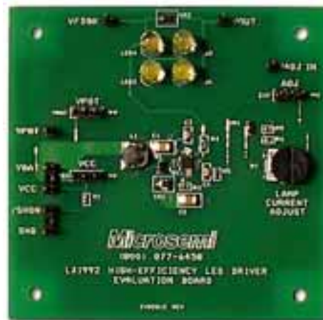
Figure 5: LX1992 Engineering Evaluation Board
