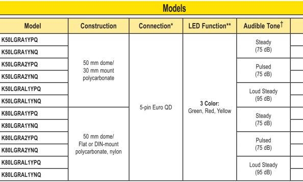
\* Integral QD models are listed. For 150 mm PVC pigtail with QD, replace Q with QP in model number (example, K50LGRA1YPQP). A model with a QD requires a mating cable (see page 3).
