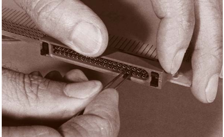
REMOVE DAMAGED CONTACT
