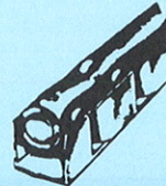
2. Insulation being pierced.
