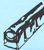
2. Insulation being pierced.
