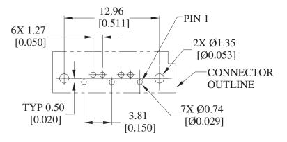
RECOMMENDED P.C.B. HOLE LAYOUT TOLERANCE ±0.05 [0.002]
