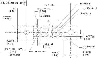
Note: Plated through holes for  $.062^{\prime\prime}$  board thickness.
