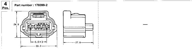
\*The color of housing is black, and that of double lock plate is yellow. \*The material of housings are of PBT with glass.
