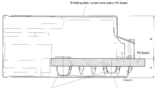
Press-in studs for mounting to PC board
