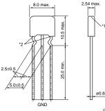
\*1 There may be a hole on the top of ferrite beads, which causes no characteristics deterioration. \*2 Bottom of the ferrite beads may not be level with each other.
