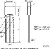
\*1 There may be a hole on the top of ferrite beads, which causes no characteristics deterioration. \*2 Bottom of the ferrite beads may not be level with each other.
