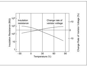
■Temperature Characteristics of Varistor Voltage - Insulation Resistance (VFS9V)
