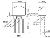
\*1 Coating extending on leads does not exceed the tangent line. Exposed electrode, if any, is covered by solder, etc.
