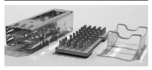
Tyco Electronics introduced an SFP system incorporating a riding heat sink to help manage excess heat when using SFP modules. This is especially suited for use with higher wattage transceivers, such as long reach applications like Dense Wavelength Division Multiplexing (DWDM).
