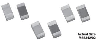
Thin Film Mil chip resistors feature all sputtered wraparound termination for excellent adhesion and dimensional uniformity. They are ideal in applications requiring stringent performance requirements. Established reliability is assured through 100 % screening and extensive environmental lot testing. Wafer is sawed producing exact dimensions and clean, straight edges.
