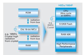
Using our 16/32-bit microcontrollers, our customers are able to tackle most of those design tasks, which developers face today. The high memory and peripheral integration allows to switch legacy multi-chip systems to singlechip, thus making systems smaller, light weight, lower power, more reliable and fast to build. Furthermore, where external busses can be removed, radiation can be greatly reduced.
