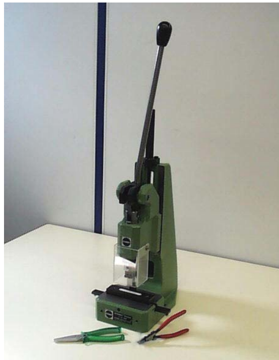
Figure 17 -- Connector Removal tooling HM2Y350
