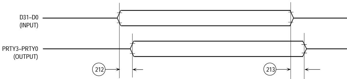
Figure 10-37. External MC68030/MC68360 Parity Bits Timing Diagram
