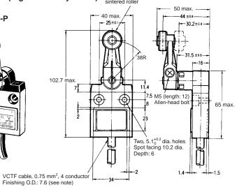
Note: S-FLEX VCTF Cables are used for weatherresistant models (D4C-P).
