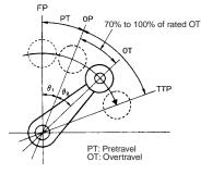
• The movement distance of the dog based on the optimum stroke is expressed by the following formula.
