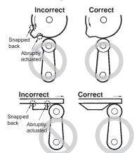
Appropriate force must be imposed on the actuator by the cam or dog in both rotary operation and linear operation. If the dog touches the lever as shown below, the operating position will not be stable.
