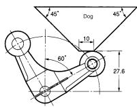
**Note:** Design the shape of the dog so that it does not come in contact with the other roller lever when the actuator is inverted.
