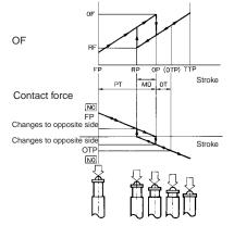
If the Limit Switch is used so that the actuator is constantly pressed, it will fail quickly and reset faults may occur. Inspect the Limit Switch periodically and replace it as required.
