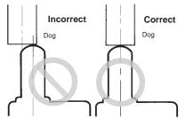
• Be sure to use the Limit Switch according to the characteristics of the actuator. If a roller arm lever actuator is used, do not attempt to actuate the Limit Switch in the direction shown below.
