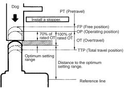
The Limit Switch may soon malfunction if the OT is excessive. Therefore, adjustments and careful consideration of the position of the Limit Switch and the expected OT of the actuator are necessary when mounting the Limit Switch.
