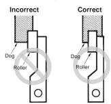
• With a roller actuator, the dog must touch the actuator at a right angle. The actuator or shaft may deform or break if the dog touches the actuator (roller) at an oblique angle.
