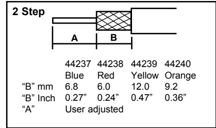
Stepped Stripping Depth For Reduced Friction
