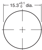
Panel Cutout Dimension Panel thickness = 1 to 4 mm
