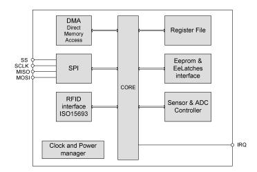
The SPI and RFID communication ways can be used concurrently. The *Core transaction arbiter* handles the priorities and the interrupts. It updates some status bits that may be used by the external microcontroller or the RFID base-station to optimize the communication.
