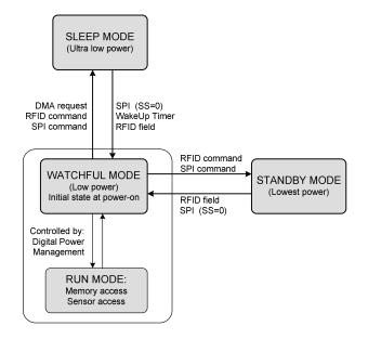
The Digital Controller can not exit this mode by itself. It can only exit it by an external interrupt: emission of a RFID field or asserting low the Slave Select input of the SPI (during a specified time)
