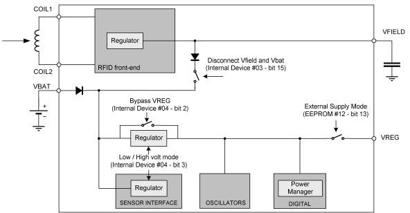
The power management mode is defined by several switches configurable through the EEPROM and EE-Latch.
