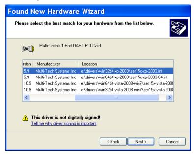
Select the top choice, e:\drivers\win32bit-xp-2003\ser15x-xp-2003.inf for Windows 32-bit Operating System; or select the second choice for Windows 64-bit Operating System e:\drivers\win64bit-xp-2003\ser15x-xp-2003-64.inf.
