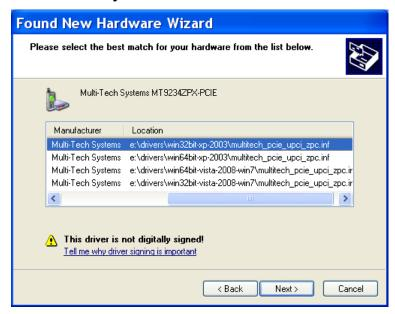
Select the top choice, e:\drivers\win32bit-xp-2003\multitech\_pcie\_upci\_zpc.inf for Windows 32-bit Operating System; or select the second choice for Windows 64-bit Operating System e:\drivers\win64bit-xp-2003\multitech\_pcie\_upci\_zpc.inf.
