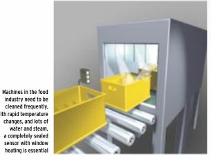
Thanks to the optic link, the sensor can be remotely set and checked while it is operating in an area where access is restricted
