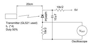
In the above figure, the transmitter should be set so that the output VouT (P-P) can be 40mV. However, the PD49PI to be used here should be of the short-circuit current Isc=2.6  $\mu$  A at Ev =100 Ix. (E<sub>V</sub> is an illuminance by CIE standard light source A (tungsten lamp).)
