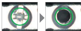
Based on the change in brightness, the presence of a screw (OK or NG) is determined.
