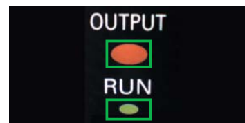
LED illumination is determined based on the area of extracted color.
