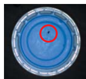
Almost indistinguishable scratches can be detected after enhancing contrast using the color filter.
