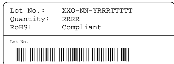
Figure 20: First label on reel: XX = Sensor Type (25 for SHT25), O = Output mode (0 = Digital), NN = Chip Version, Y = last digit of year, RRR = number of sensors on reel divided by 10 (200 for 2000 units), TTTT = Traceability Code.
