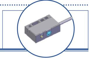
The OPB720 is a reflective switch designed to detect objects as far away as 24" (610 mm). Detectable object sizes can be as small as 0.08" (2mm) at a distance of 8" (20 mm). The OPB720 has a logical output that switches from a high level with no reflection target to a low level with a reflection target. With the addition of hysteresis, the OPB720 minimizes switching oscillations on the output. The open collector output transistor and power requirements is compatible with most PLC's
