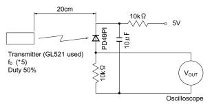
In the above figure, the transmitter should be set so that the output V<sub>OUT (P-P)</sub> can be 40mV. However, the PD49PI to be used here should be of the short-circuit current Isc=2.6  $\mu$  A at Ev =100 lx. (Ev is an illuminance by CIE standard light source A (tungsten lamp).)
