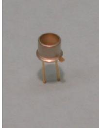
BONDS [12.70] MIN 45 C 589 Ø0.210[5.33] 0.100[2.54] VIEWING କୁ ANGLE 0.042 ANODE HEADER Ø0.018[0.46] PHOTODIODE CATHODE Ø0.018[0.46] 0.068[1.73] SQUARE 0.059[1.50] SQ ACTIVE AREA **TO-46 HERMETIC CAN PACKAGE** ACTIVE AREA =  $2.03 \text{ mm}^2$
