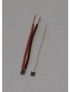
Photoconductive Type PDB-C603 Photovoltaic Type PDB-V603
