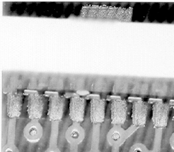
Picture 1. Castellations misaligned to land pads in X-axis before reflow.
