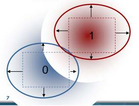
Si4706/49 RDS decoder extends acceptance region using advanced on-chip processing
